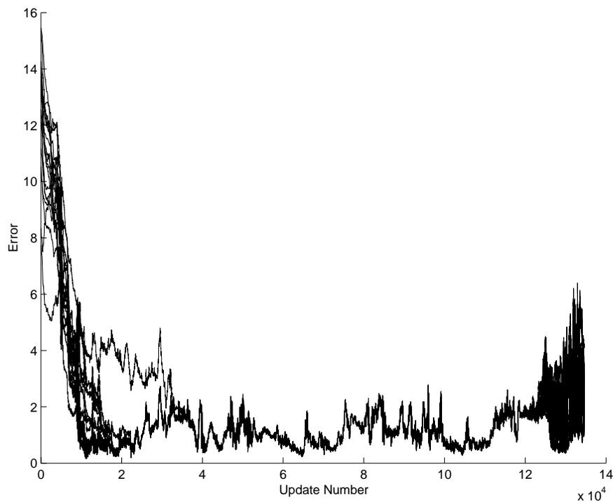
**Fig 15:** Convergence curves for a matched Natural Gradient Algorithm under Random Channel Conditions
