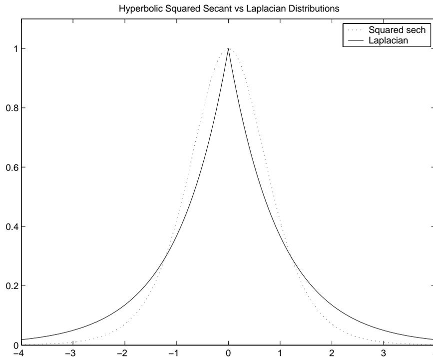
**Figure 8:** Comparison of Laplacian and  $\text{sech}^2 u$  distributions
