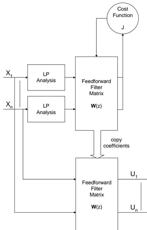
**Fig 12:** Equivalent ICA architecture without residual reconstruction artefacts
