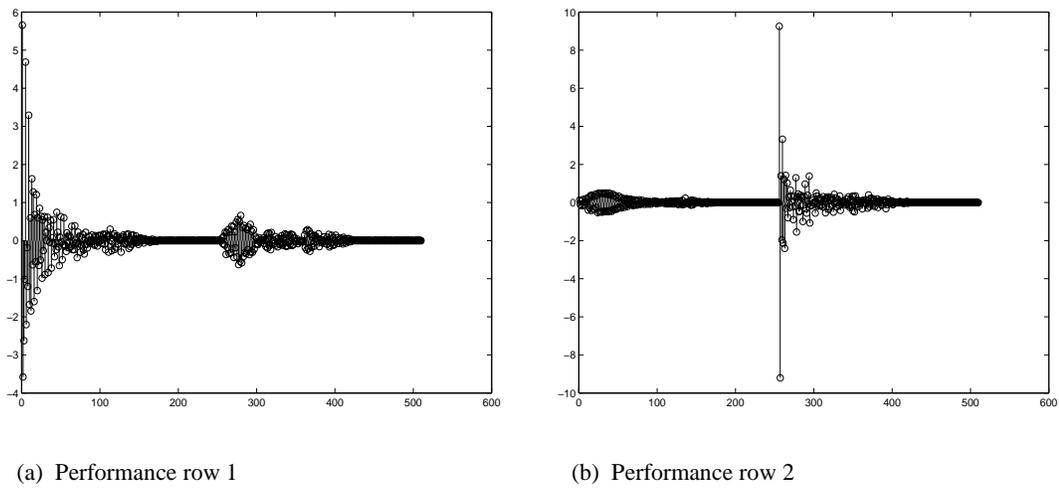
**Fig 23:** Final impulse responses of the filters in  $\mathbf{P}(z)$ . Each row contains two filters, the impulse responses which are concatenated.
