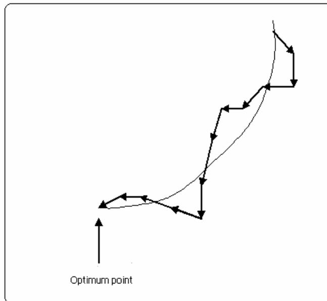
**Figure 3:** An illustration of the locus of a deterministic gradient (solid line), and stochastic gradient (arrowed line)
