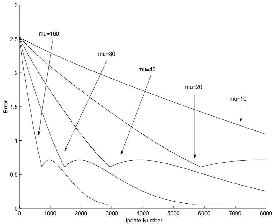
**Fig 17:** Error curve of multiple decorrelation algorithm on two mixed voices with changing gradient step-size
