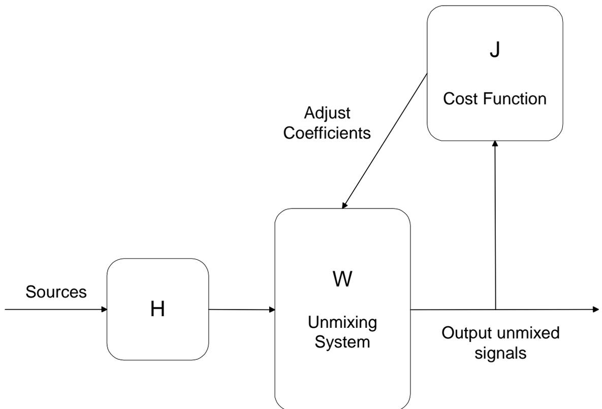
**Figure 2:** Block Diagram of a Separating System
