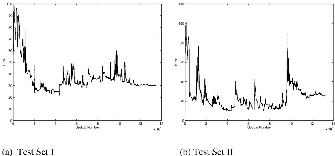
**Fig 21:** Error curves for the separation of two mixed voices in the Infomax feedback architecture
