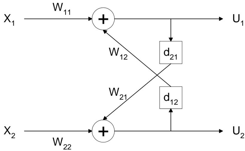
**Figure 4:** A feedback separation network with adaptive weights and delays
