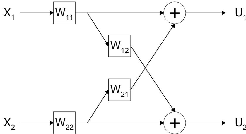
Figure 6: A feedforward matrix of filters
