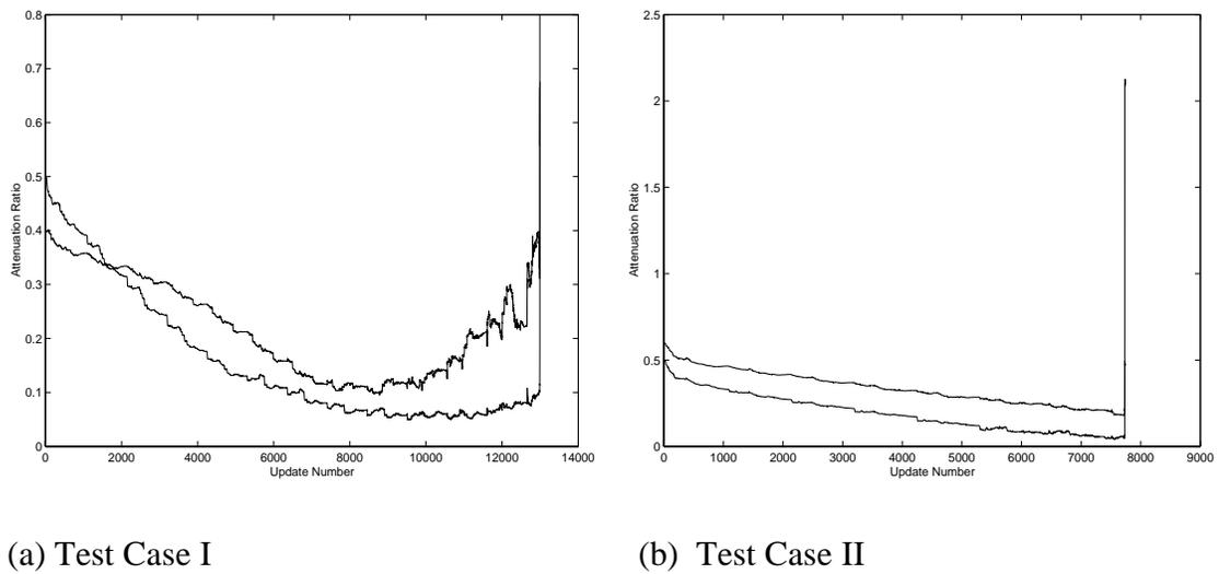
**Fig 26:** Channel attenuation ratios for the feedforward architecture.
