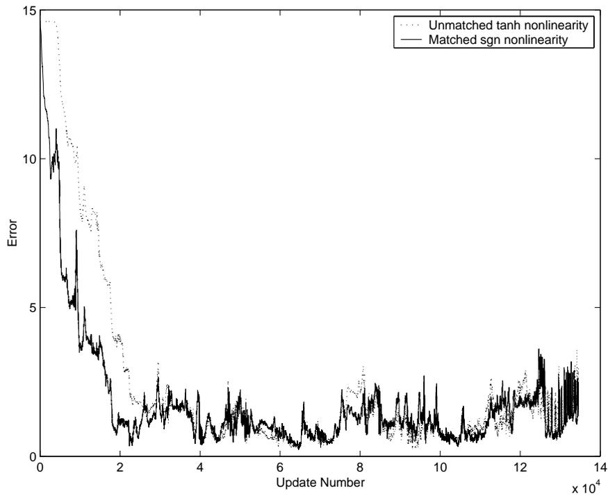
**Figure 14:** Comparison of convergence curves with unmatched sigmoidal and matched Laplacian nonlinearities
