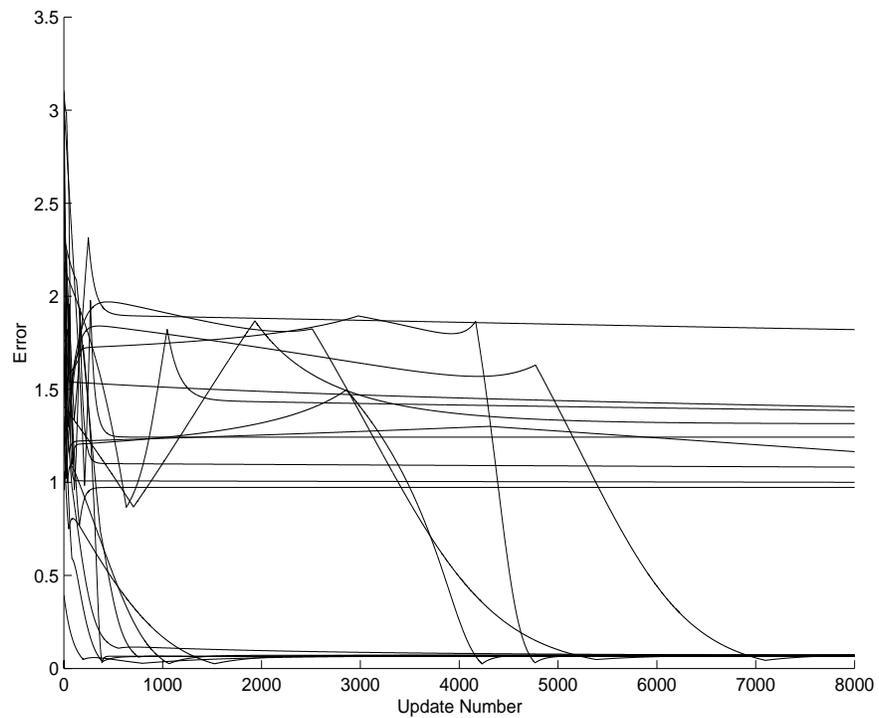
**Fig 18:** Error curves of multiple decorrelation algorithm for two mixed voices under random channel conditions
