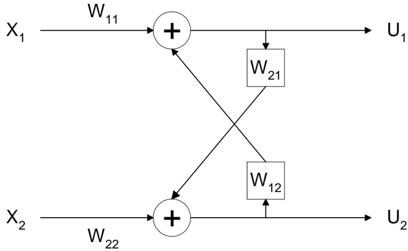
Figure 5: A feedback separation network employing adaptive cross filters
