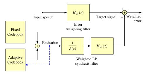
Fig. 7 Restructured Analysis-by-Synthesis Coding
