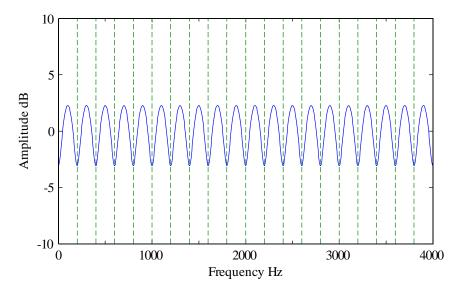
Fig. 5 Harmonic noise weighting filter response ( $g_{HNW} = 0.2, L = 40 (200 \text{ Hz})$ ).
