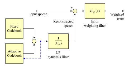
Fig. 6 Analysis-by-synthesis coding.
