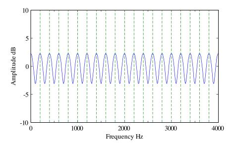
Fig. 12 Pitch postfilter ( $g_{ppf} = 0.1875$ , L = 40 (200 Hz)).
