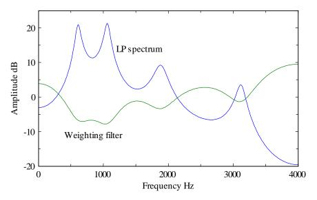
Fig. 4 Formant weighting filter response.
