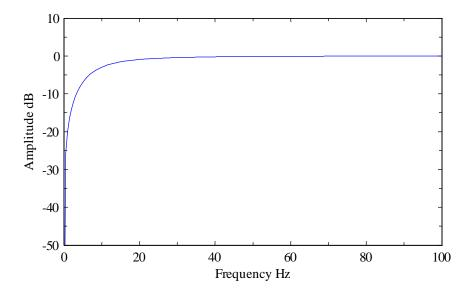
Fig. 2 Highpass filter frequency response.
