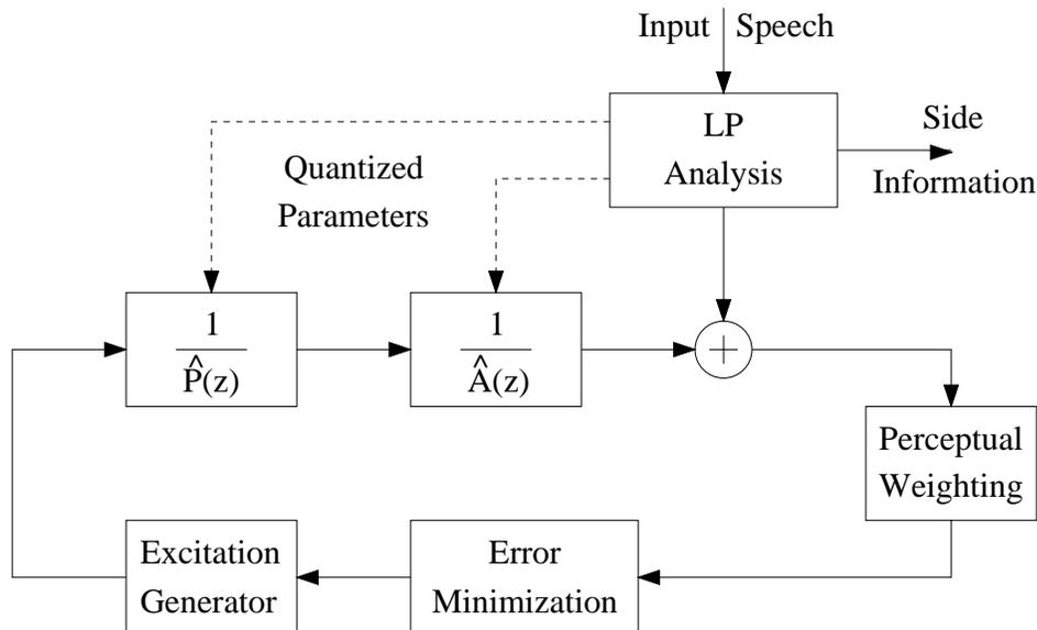
Figure 1.2: Linear predictive based analysis-by-synthesis (LPAS) coder.
