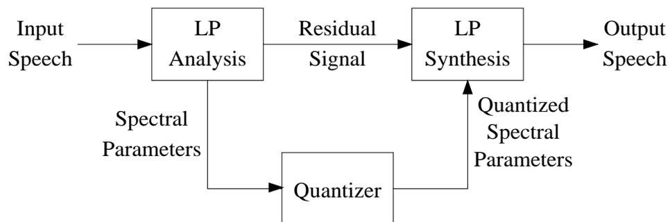
Figure 2.3: Simulation environment for speech spectral codec evaluation.
