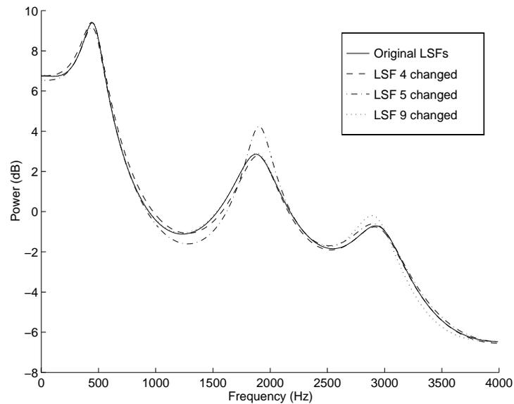
Figure 2.2: Effect of changing a LSF value on the LP spectrum. In the first altered plot, the 4-th LSF is changed from 1315 Hz to 1275 Hz. In the second altered plot, the 5-th LSF is changed from 1745 Hz to 1800 Hz. In the third altered plot, the 9-th LSF is changed from 3025 Hz to 2995 Hz.
