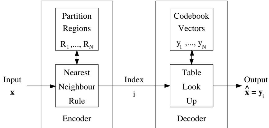
Figure 3.3: Model of a Vector Quantizer.
