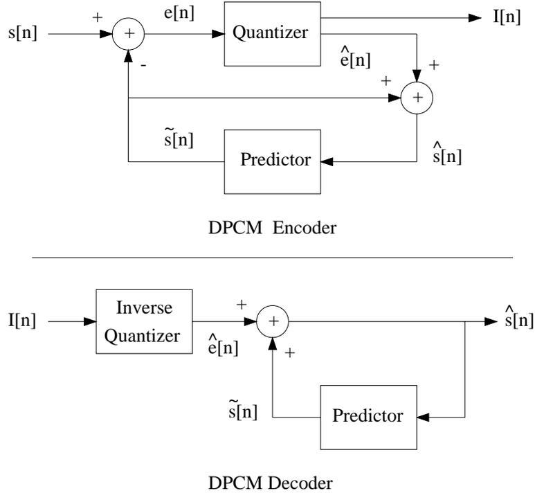
Figure 1.1: Differential pulse code modulation (DPCM) coder.
