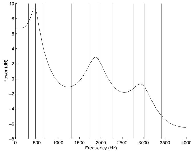
Figure 2.1: LP spectrum with LSF positions superimposed.
