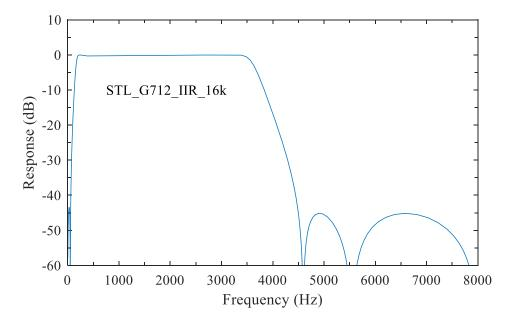
Fig. 6 PCM (G.712) filter response.
