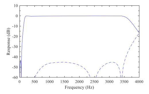
**Fig. 7** PCM (G.712) filter response with 8 kHz sampling. The dashed line shows the aliased response
