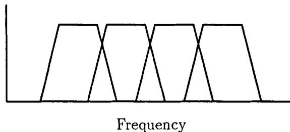
**Fig. 1.2** Filter characteristics with spectral overlap
