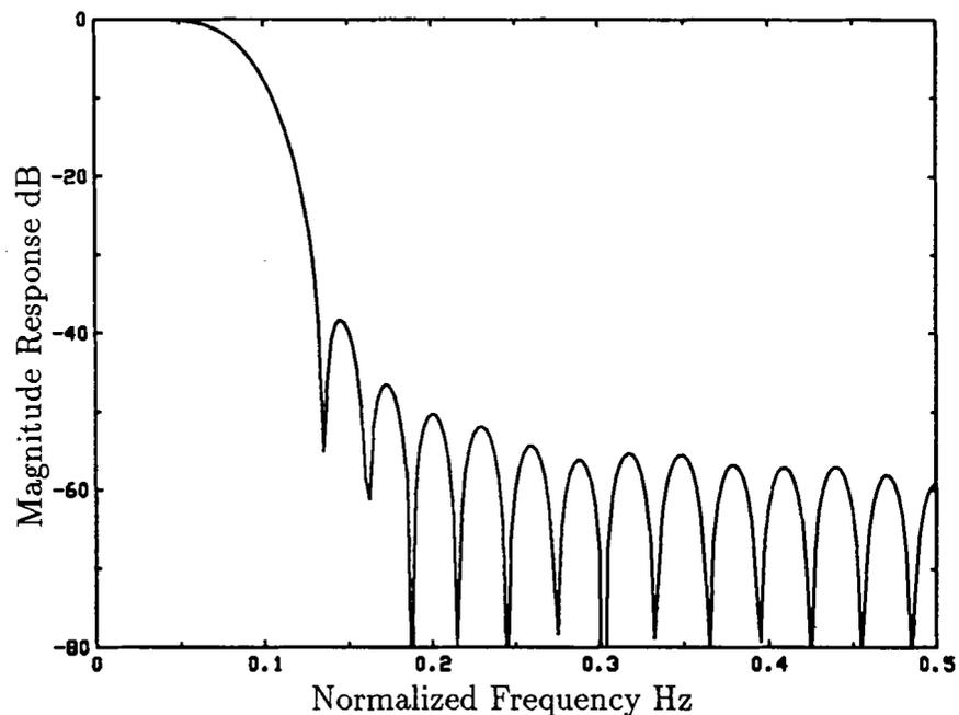
**Fig. 5.1** Magnitude response of the lowpass filter for system T1. The weighting factors are  $(\gamma_1, \gamma_2, \gamma_3, \gamma_4) = (100, 1, 1, 0.01)$ .
