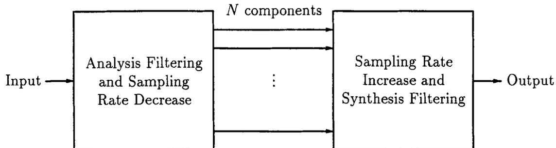
**Fig. 1.3** General illustration of a subband system
