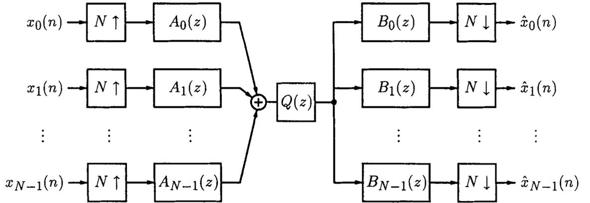
**Fig. 6.1** Channel distortion in a transmultiplexer
