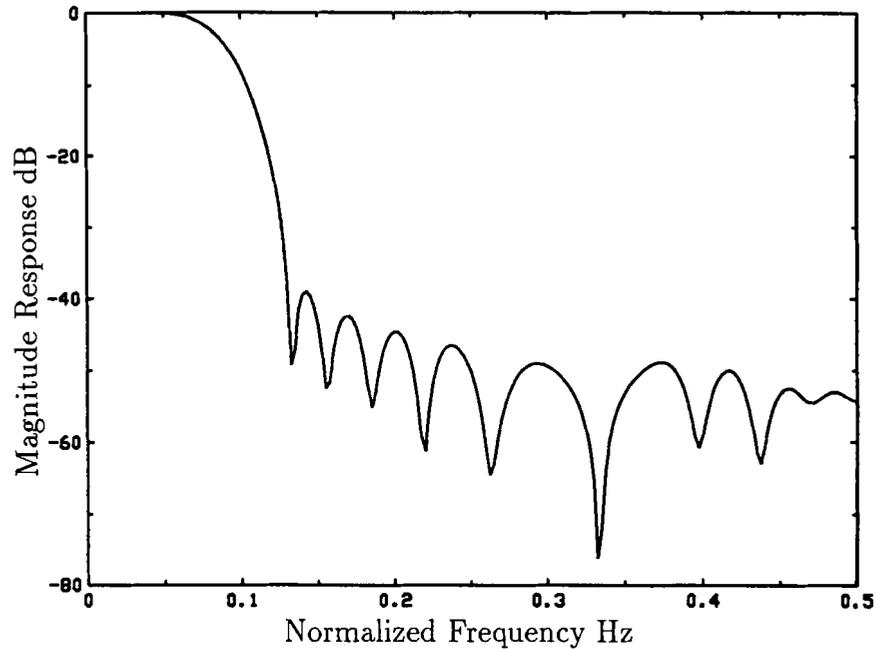
**Fig. 5.2** Magnitude response of the lowpass filter for system T3.
